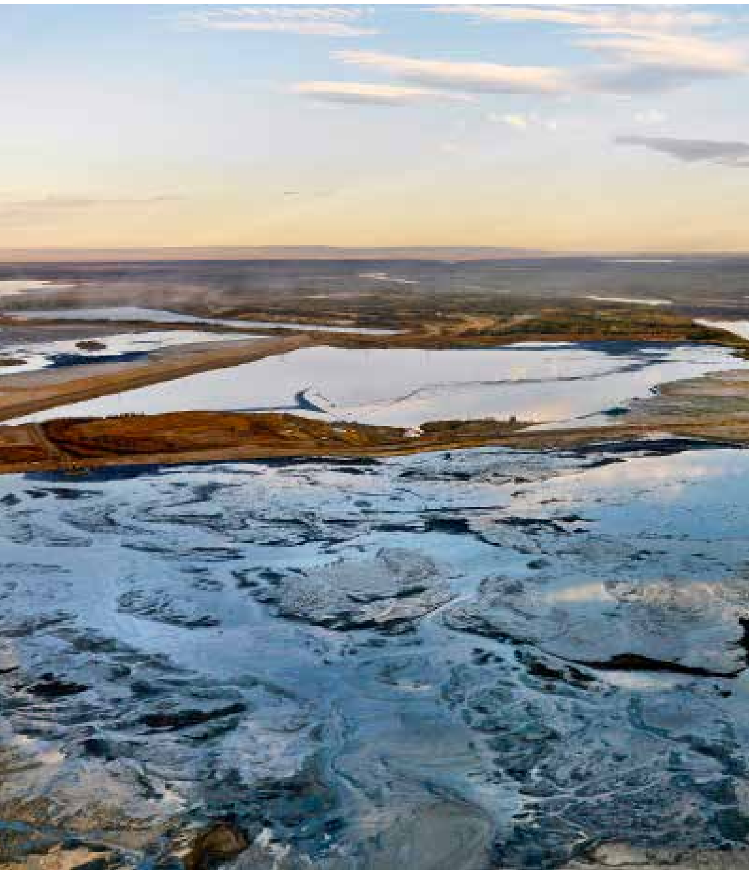
Tar-sands field, Alberta: Only about 20 percent of the deposits are within seventy-five meters of the surface, so the extraction process utterly transforms the landscape. Here, the massive tailings pond is in the foreground, with the upgrader facilities of Syncrude and Suncor in the background.
